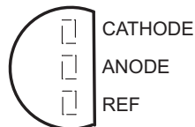
TL431, TL431A, TL431B . . . LP (TO-92/TO-226) PACKAGE (TOP VIEW)
