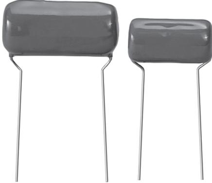
Type 716P ORANGE DROP® is a high performance version of the popular Type 715P. It is made from polypropylene and foil with copper leads for the ultimate in high pulse current and high rms current capability. It is a pressed unit for better utilization of board space.
