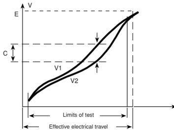
It is the maximum deviation between the actual voltage outputs of 2 or more pot modules in the same assembly. It is expressed as a percentage of the total applied voltage, or preferably in dB attenuation.
