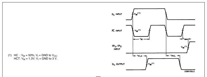
Fig.9 Waveforms showing the parallel load input  $(\overline{PL})$  and data  $(D_n)$  to  $Q_n$  output propagation delays and  $\overline{PL}$  removal time to clock input  $(CP_U, CP_D)$ .
