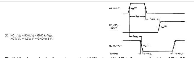
Fig.10 Waveforms showing the master reset input (MR) pulse width, MR to  $Q_n$  propagation delays, MR to  $CP_D$ , removal time and output transition times.
