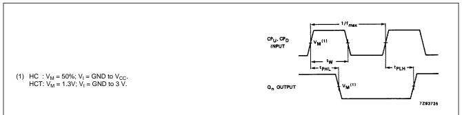
Fig.7 Waveforms showing the clock  $(CP_U, CP_D)$  to output  $(Q_n)$  propagation delays, the clock pulse width, and the maximum clock pulse frequency.
