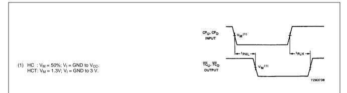
Fig.8 Waveforms showing the clock (CP<sub>U</sub>, CP<sub>D</sub>) to terminal count output ( $\overline{TC}_U$ ,  $\overline{TC}_D$ ) propagation delays.
