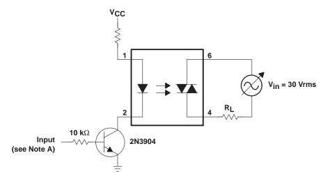
NOTE A. The critical rate of rise of off-state voltage, dv/dt, is measured with the input at 0 V. The frequency of V<sub>in</sub> is increased until the phototriac turns on. This frequency is then used to calculate the dv/dt according to the formula:
