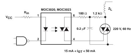
Figure 7. Inductive Load With Nonsensitive-Gate Triac
